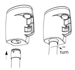
12. Insert the nozzle into the console. The installation of the WallyFlex is now completed.
