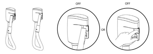
**Note:** When in use, for increased safety, the central vacuum unit can be stopped at any time, simply by pressing the switch on the WallyFlex console.
