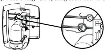
6. Then, fix the console onto its mounting plate with the three short screws (#10 3/4").
