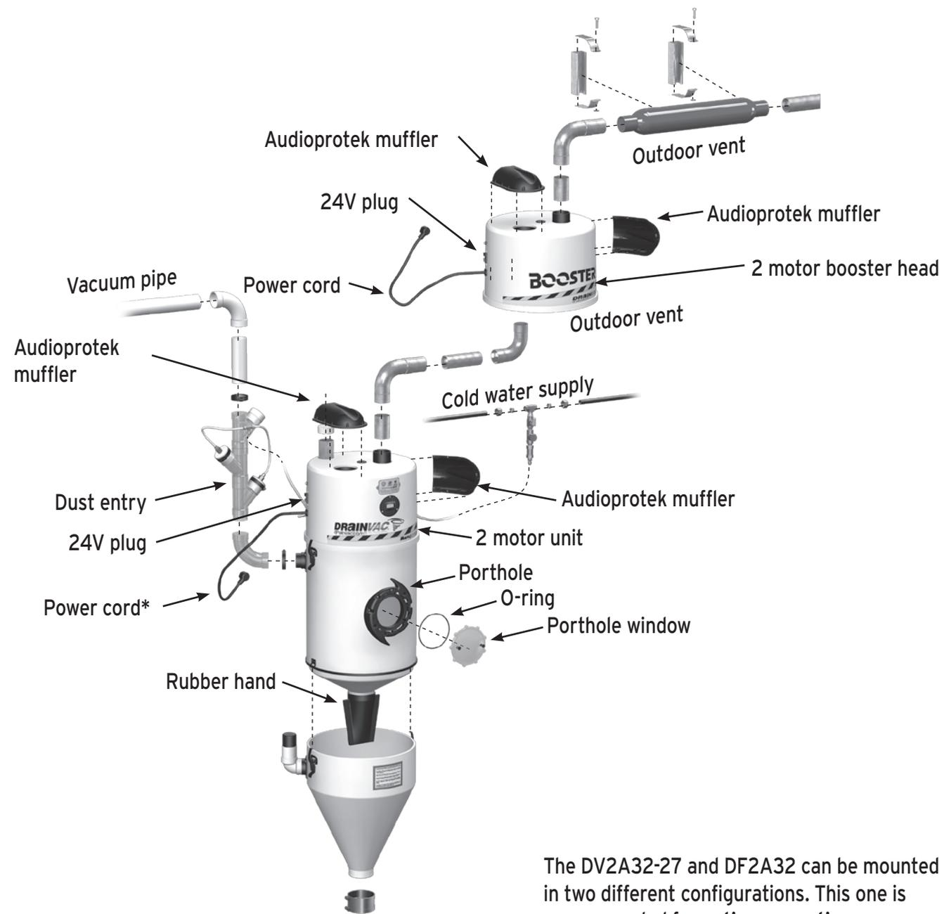
The DV2A32-27 and DF2A32 can be mounted in two different configurations. This one is recommended for **optimum suction power**.
