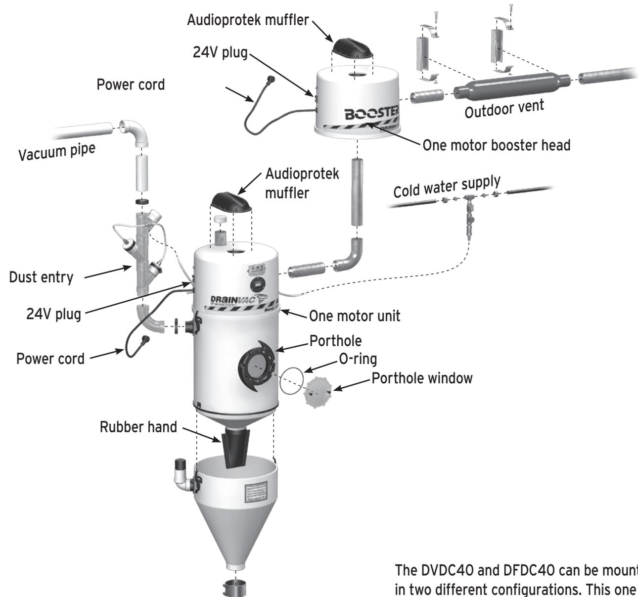
The DVDC40 and DFDC40 can be mounted in two different configurations. This one is recommended for **optimum suction power**.
