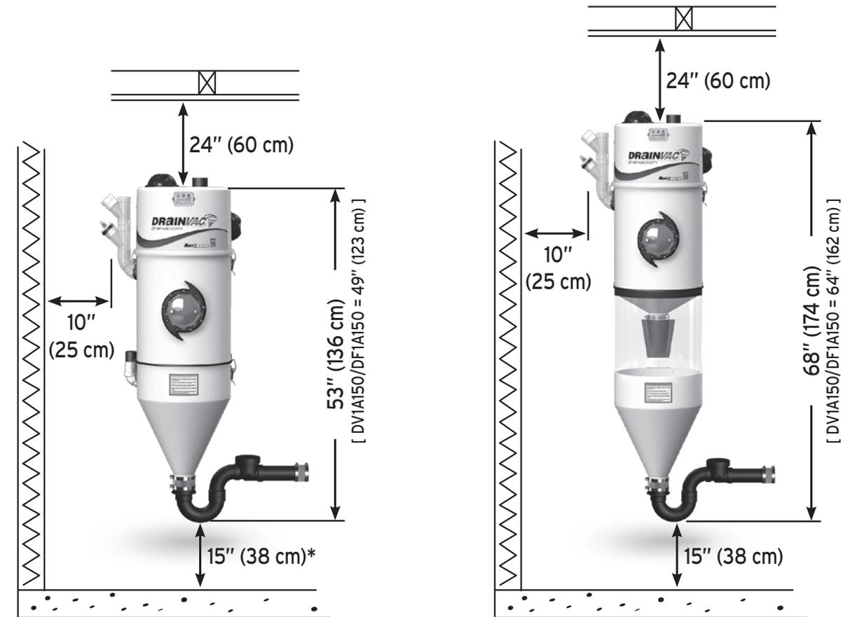
\* For **compact** models, the bottom of the P-Trap can be installed at 15" (38cm) from the floor. However, we recommend **26" (66 cm)**, if possible, so that a pail can be placed under the unit, if need be, when removing the P-Trap.
