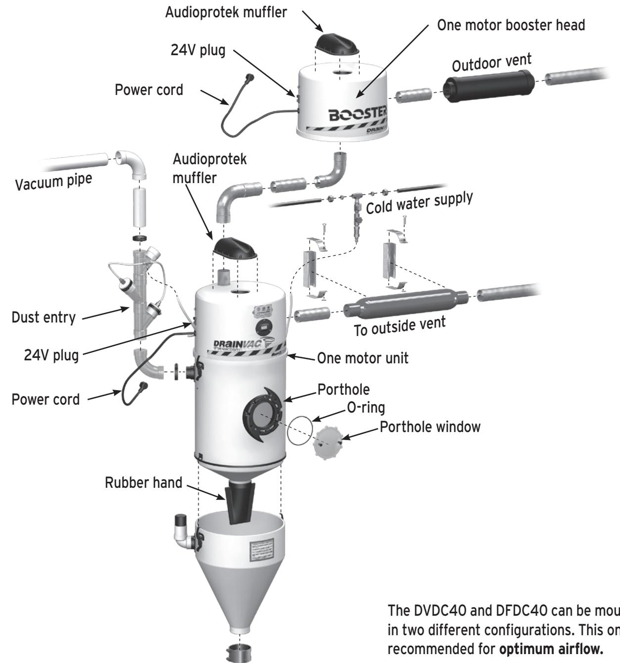
The DVDC40 and DFDC40 can be mounted in two different configurations. This one is recommended for **optimum airflow**.
