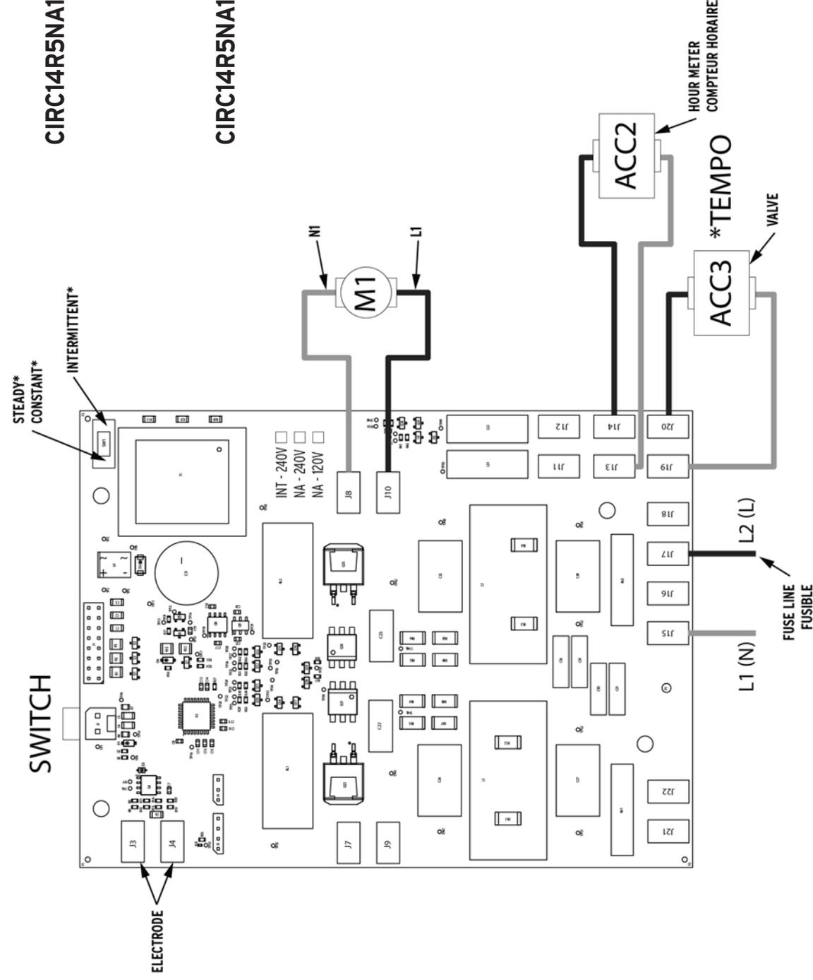
**\*STEADY: COMMERCIAL DEFAULT SETTING - CONTINUOUS WATER FLOW**
