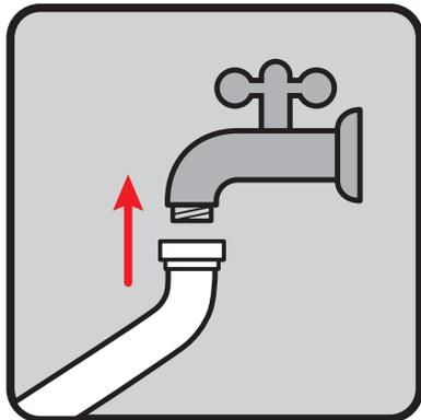
Connect the water hose from, either the cleaning tool or cleaning wand, to the faucet.
