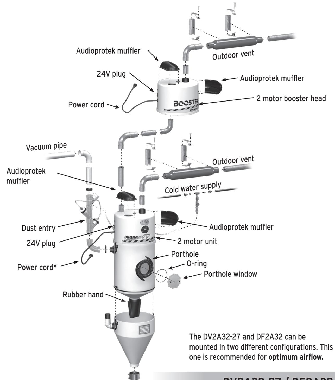
The DV2A32-27 and DF2A32 can be mounted in two different configurations. This one is recommended for **optimum airflow**.
